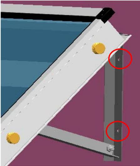
Note: For double collectors, please assemble the other collector same as Step 1 to Step 3. And keep the distance between two collectors to be 60cm at least (also need consider the length of PEX Black Pipe). As picture.
