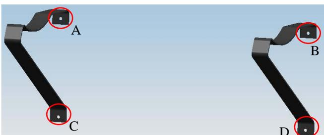
Note: to make sure both Boiler Support A be vertical to the ground.
